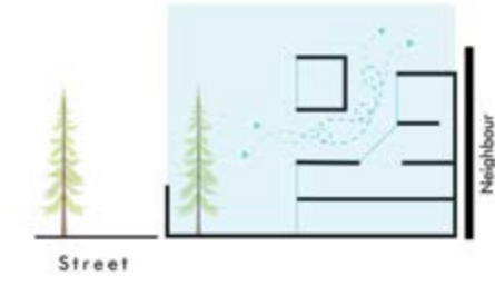
Ventilation Through Void
