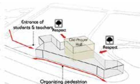
Considering the access of passengers and respect to old trees, the parts of the volume have been removed
